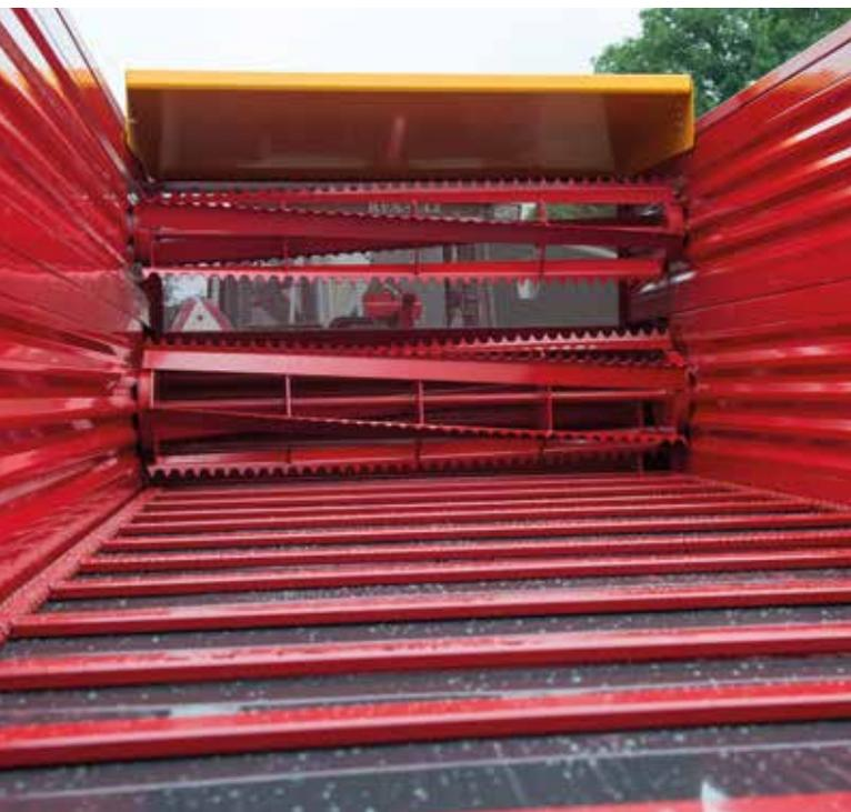
The Feedo's are fitted with two or more open and aggressive silage beaters. The beaters have different diameters and run at different speeds as standard. In this way an outstanding distribution and mixing of the different sorts of silage and feed are guaranteed. The beaters are mechanically driven from the power takeoff (PTO). Due to the special Feedo forage box-feeder beaters the feed is distributed evenly and without structure loss, whereupon it will be discharged by the cross-conveyor.
